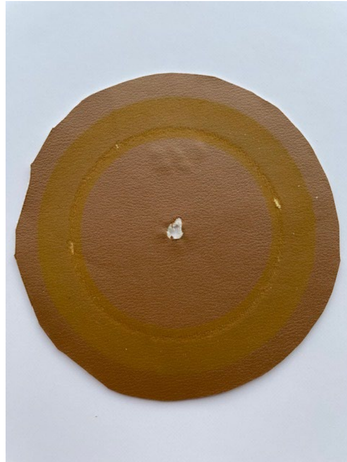
Competitor silicone 250 revolutions - FAIL Note severe abrasion and tackiness
