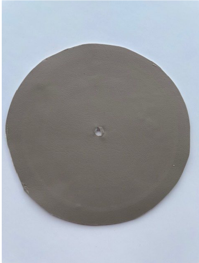
envirosil 750 revolutions - PASS Note lack of abrasion Note no tackiness
